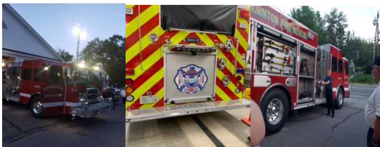
Engine 2 is designed to be a “Rescue/Pumper” which allows enough compartment space to carry firefighting equipment and rescue equipment like extrication and stabilization tools.
